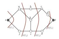
$$\begin{array}{lcl} \delta(U_1) & = & \{sa, sj\} \\ \delta(U_2) & = & \{ab, ah, ji\} \\ \delta(U_3) & = & \{bc, hc, ig\} \\ \delta(U_4) & = & \{dt, gt\} \end{array}$$
