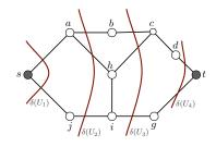
$$\begin{array}{rcl} \delta(U_1) & = & \{sa, sj\} \\ \delta(U_2) & = & \{ab, ah, ji\} \\ \delta(U_3) & = & \{bc, hc, ig\} \\ \delta(U_4) & = & \{dt, gt\} \end{array}$$
