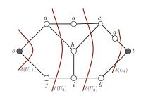
$$\begin{array}{lcl} \delta(U_1) & = & \{sa, sj\} \\ \delta(U_2) & = & \{ab, ah, ji\} \\ \delta(U_3) & = & \{bc, hc, ig\} \\ \delta(U_4) & = & \{dt, gt\} \end{array}$$
