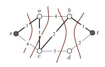
$$\begin{array}{rcl} U_1 & = & \{s\} \\ U_2 & = & \{s,a\} \\ U_3 & = & \{s,a,c\} \\ U_4 & = & \{s,a,b,c,d\} \end{array}$$
