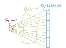
The detected projection value is in the case of a fan beam X-ray source a 1D function  $p: \mathbb{R} \to \mathbb{R}$ .
