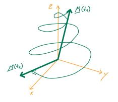
The varying magnetization can be measured using electromagnetic coils (induction principle).
